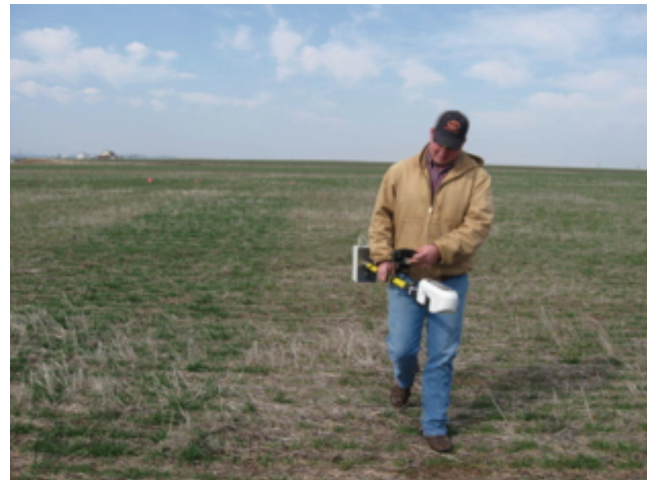
Figure 2. Farmer next to an N-Rich Strip, being sensed with a GreenSeeker™ sensor.
