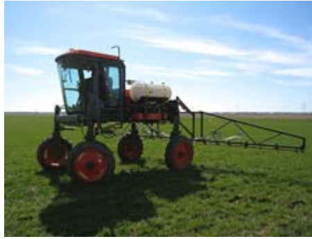
Fig. 2. High clearance applicator with a 30-ft boom used to make top-dress nitrogen fertilizer applications in winter wheat.
