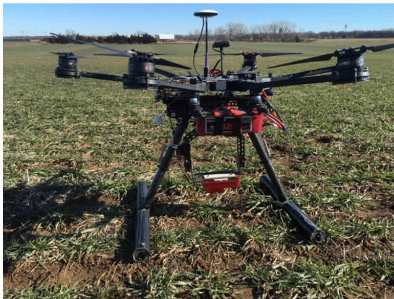
Figure 3. Using handheld Holland Scientific Rapidscan prior to topdressing wheat (top, photo by Dave Mengel, K-State Research and Extension) and MicaSense mounted to DJI S800evo prior application (bottom, photo by Ray Asebedo, K-State Research and Extension).
